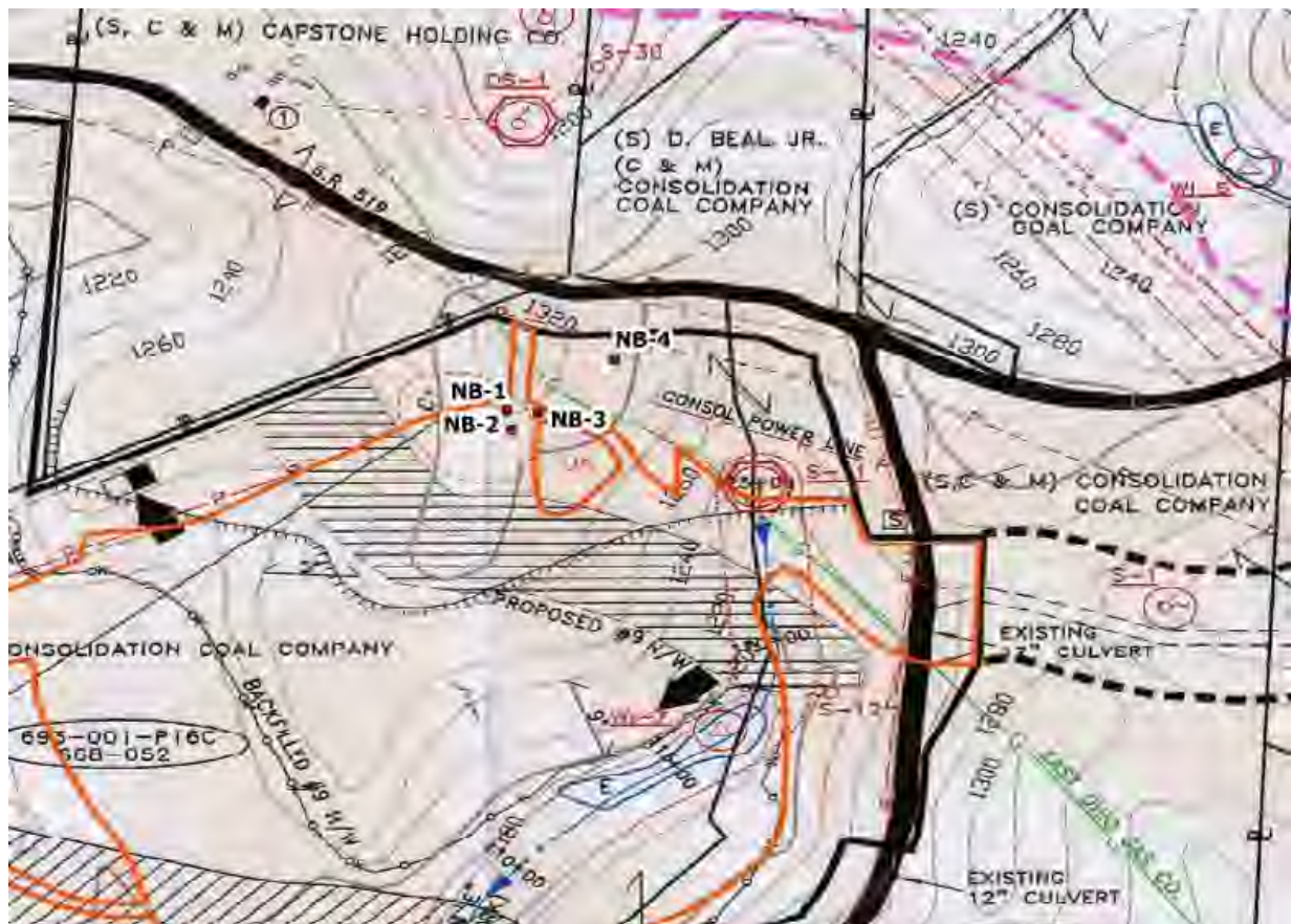
Boring Overlay – Permitted Mine Map (D-2100) Excerpt
