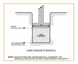
Over-excavation for granular structural fill placement below footings should be conducted as shown below. The over-excavation should be backfilled up to the footing base elevation, with describe soil type placed, as recommended in the **Earthwork** section.
