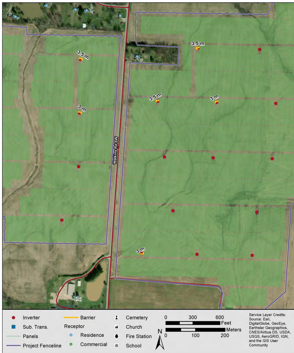
FIGURE 17: SOUND BARRIER LOCATIONS INCLUDING MODELED BARRIER HEIGHT
