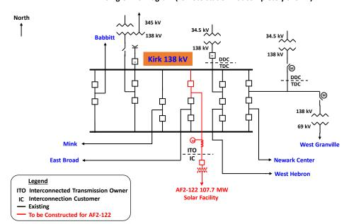
AF2-122 Point of Interconnection Kirk 138 kV Substation Single-line Diagram (remote station not completely shown)
