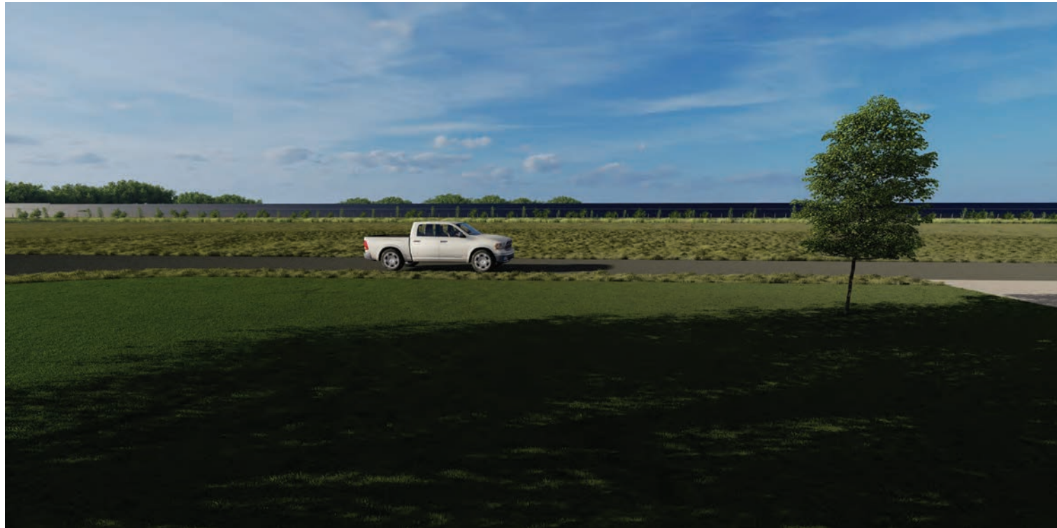
HIGH DENSITY PLANTING - POLLINATOR MIX, LARGE SHRUB / SMALL TREES AND LARGE TREES SOLAR PANELS FROM OVER A 300' DISTANCE ON A NORTH-SOUTH ROAD. PANELS SHOWN AT MAXIMUM 15' HEIGHT, 60 DEGREE TILT.
