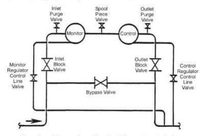
Purging Procedure for Settings Containing Self-Operated Regulators
