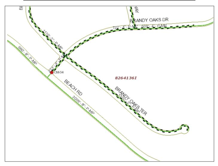
Propane Piping System Converted to Natural Gas: Normal Pressure Color Code Outlined with Black Dashes
