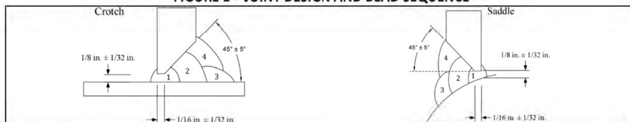
FIGURE 1 – JOINT DESIGN AND BEAD SEQUENCE
