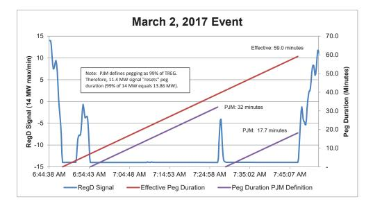
As noted in the text box within the graph, PJM's definition of pegging resets the clock when there are short releases in the Regulation signal, illustrated by the difference between the purple and red lines. As shown in this example, RegD resources are clearly being directed to operate outside of their design parameters. There are numerous occurrences in which pegging events have durations up to or approaching an hour.<sup>49</sup>
