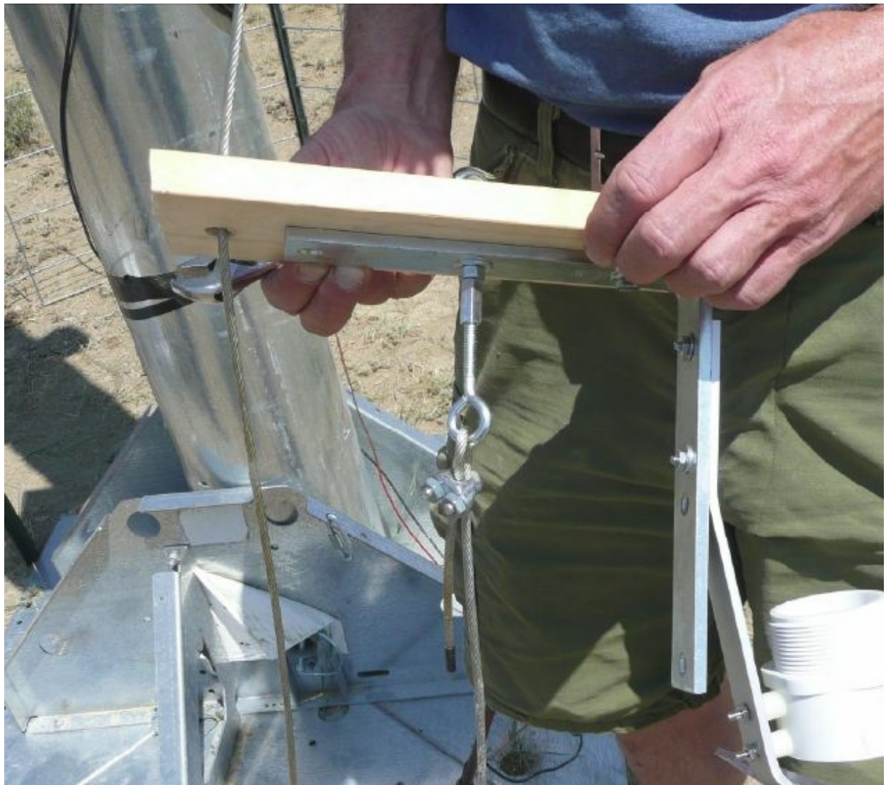
Appendix B. Bat-Hat hardware assembly used to elevate the microphone to 50-m on the met tower.
