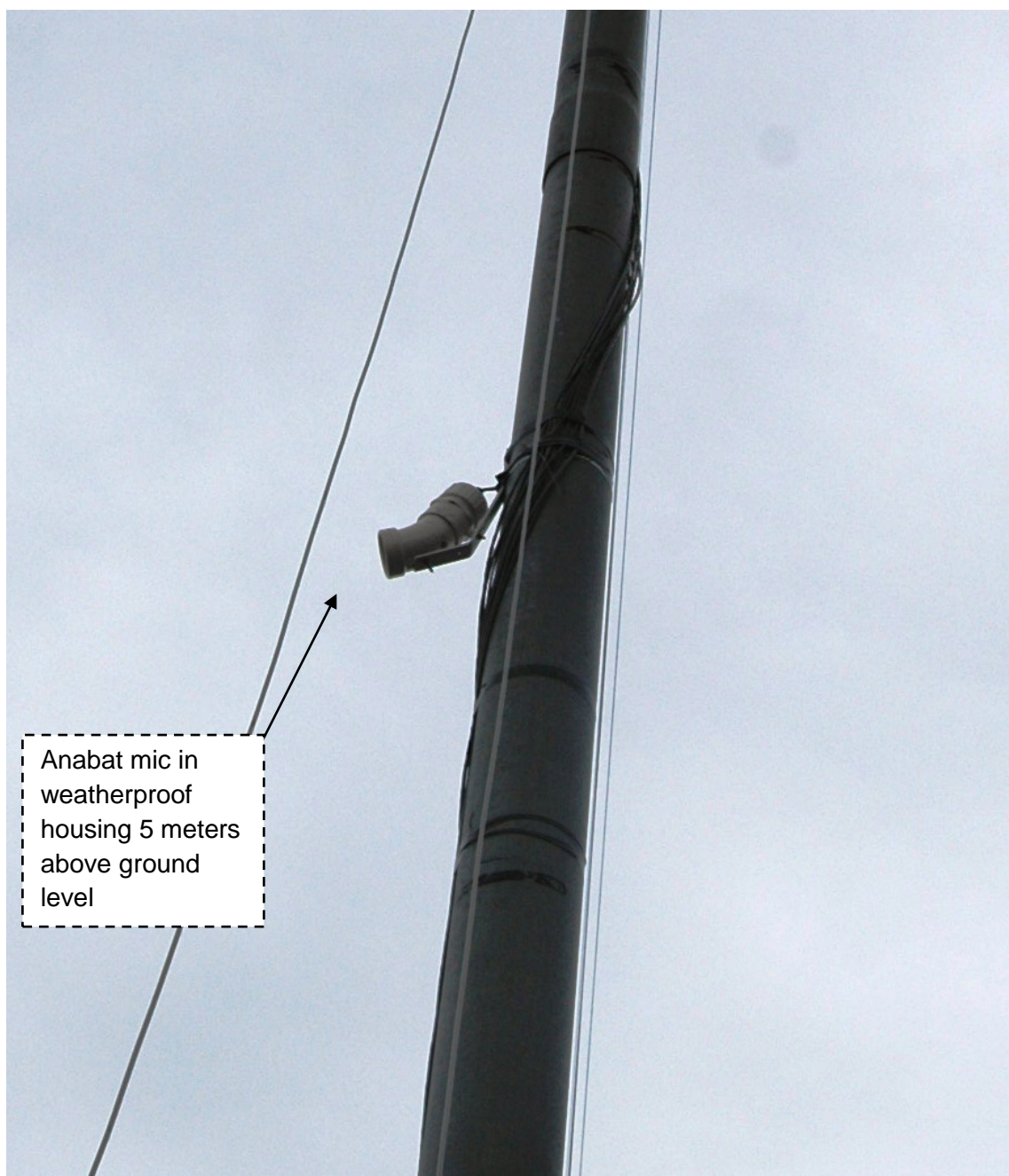
Appendix B. The 5-m Anabat setup on the met tower.
