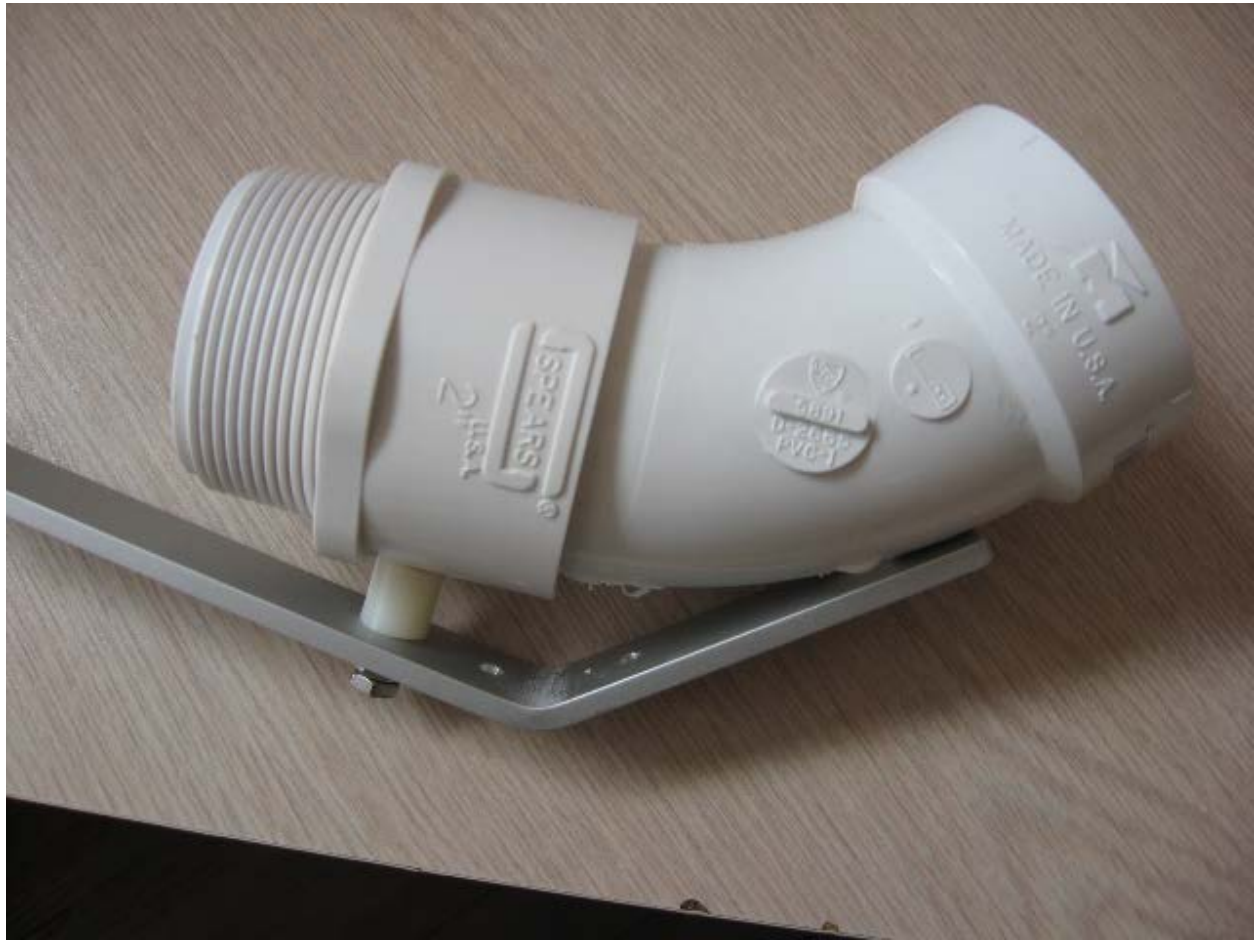
Appendix B. The 45-degree angle PVC elbow housing mount used to mount the microphone for both the 5-m and 50-m heights on the met tower.
