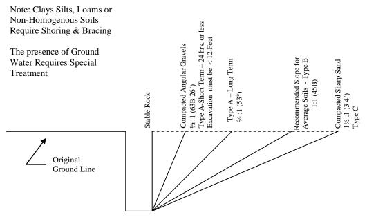
All sloping systems for excavations 5 to 20 feet in depth must be constructed under the instruction of the designated "Competent Person".
