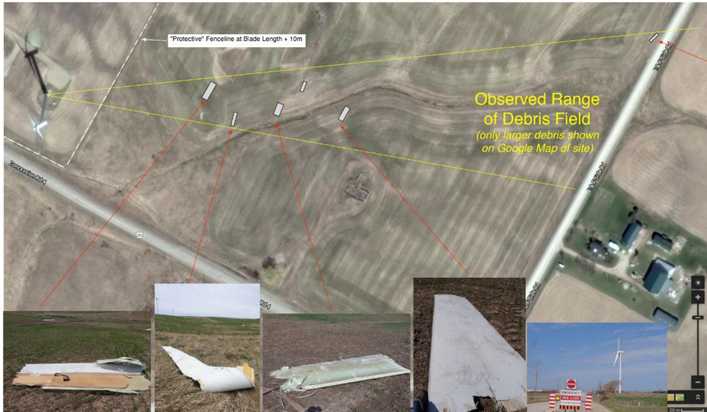
Debris at 150m from tower - 1.2m x 3.6m - Note Binoculars placed on debris for Scale
