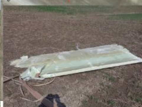
Debris at 210m from tower - 1.2m x 3.0m
