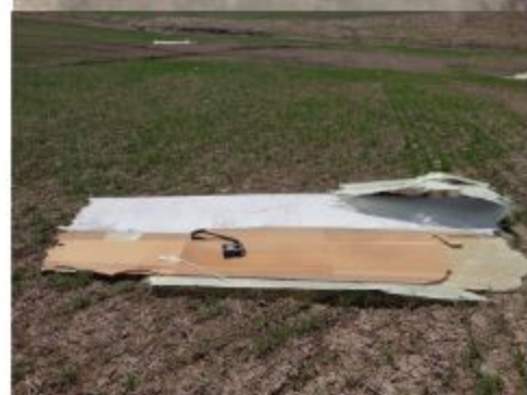
Debris at 150m from tower - 1.2m x 3.6m - Note Binoculars placed on debris for Scale
