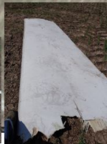
Debris at 280m from tower - 1.2m x 3.0 m - Note Boot at bottom left corner for Scale
