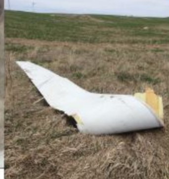
Debris at 170m from tower - 1m x 3.6m
