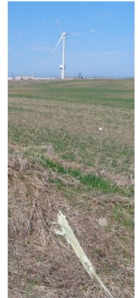
Debris at 560m from tower - 1 m x 0.15m
