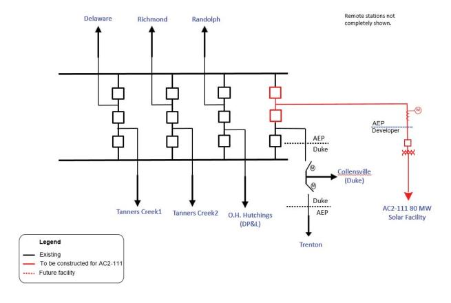
Figure 2: Point of Interconnection (College Corner 138 kV Substation)
