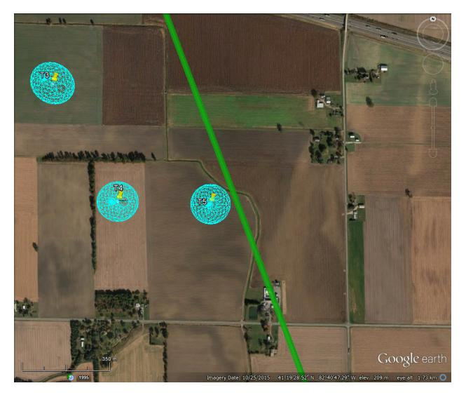
Figure 6 – Turbine 5 close to Microwave Path WQRW547/WQRW848
