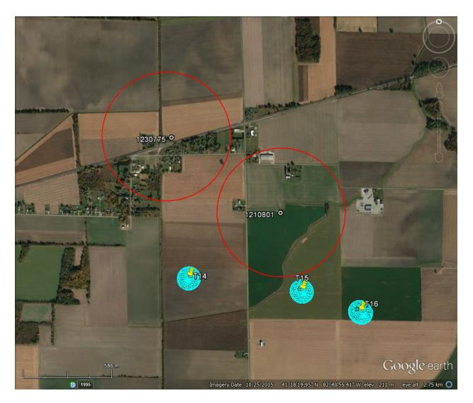
Figure 27 – Planned Turbines near FCC-Registered Towers 1210801 & 1230775
