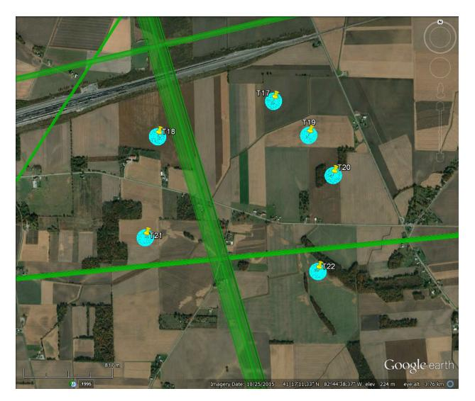
Figure 8 – Turbines 18, 21 and 22 near Microwave Paths
