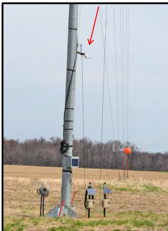
Figure 2.2. Photograph of the Low detector suspended from a specialized met tower pulley system – Republic Wind Farm, 2011. The red arrow indicates the detector location.
