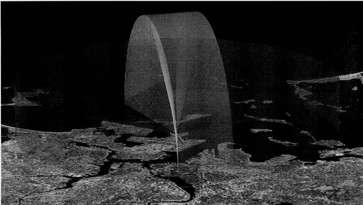
**Figure 3.** Computer representation of the potential survey volume scanned by the horizontal and vertical radars used by the U.S. Fish and Wildlife Service in spring 2012. Graphic provided by DeTect, Inc.
