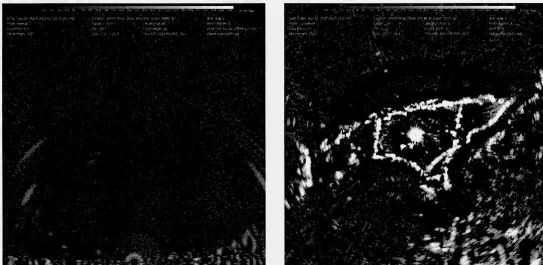
**Figure 4.** Clutter maps from vertical (left) and horizontal (right) scanning radars at study sites in Ohio and Pennsylvania during the spring 2012 migration season. Brighter areas represent static returns from stationary objects, such as tree lines and fencerows. Target detection may be obscured in these areas because of obstructions from the objects.
