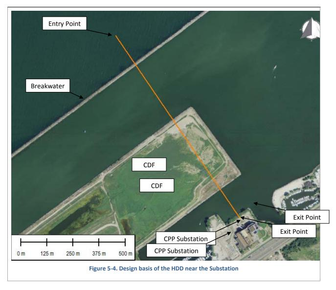
The location of the drill hole on land is determined as the 'exit point' of the power cable. The 'entry point' on the lake is where the cable will be pulled in and through to the exit point.
