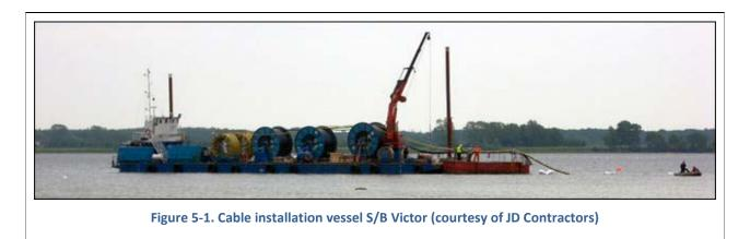
The cable likely will be delivered in two lengths, one for the export cable and one for the inter-array cables. The inter-array cable will be cut at appropriate locations in the field for each individual interarray cable length. The total length of the cable is approximately 20 km. Jointing in the field is not necessary; although, depending on the cable supplier, field joints may be required (see Section 6.
