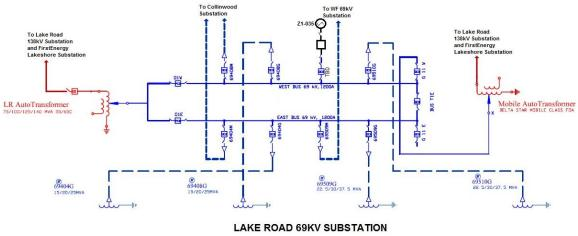
Figure 1. One Line Diagram
