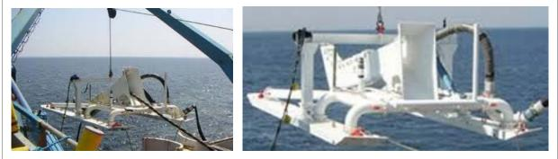
Figure 5-2. Oceanjet 200 Jetting Sled trencher
