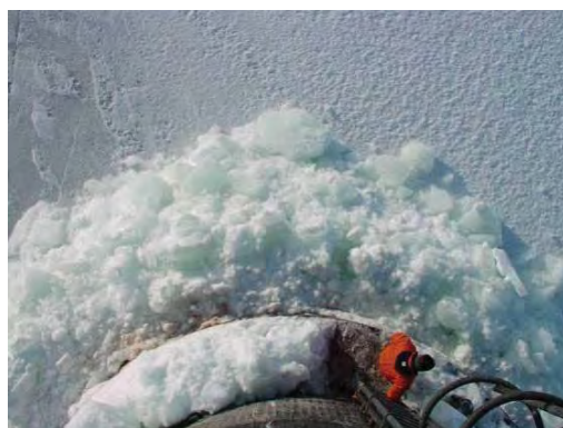
Figure 6-38: Crushing Failure on Vertical Structure
