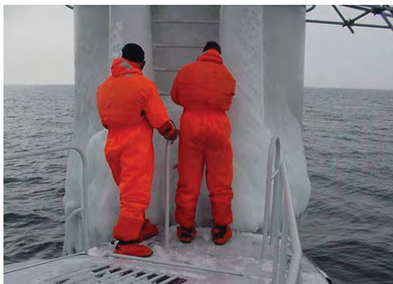
Figure 7-10: Ice Formation on Access Ladder
