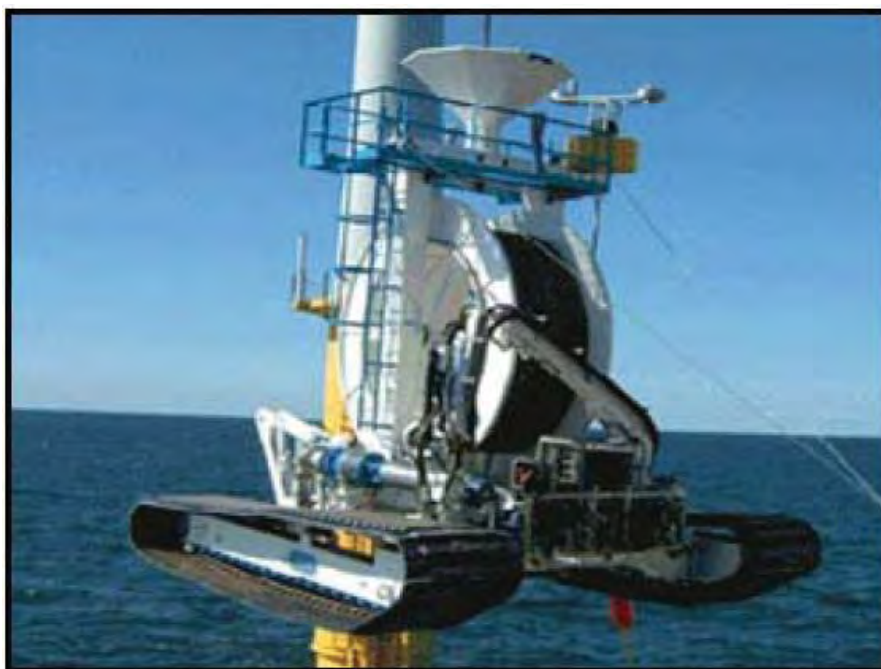
Figure 8-19: Combined Subsea Array Cable Laying and Burial Machine
