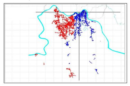
**Figure 3-4:** The extent of propane flow into the northern Kentucky part of the system from the Kentucky propane-air peaking plant at peak demand flow.
