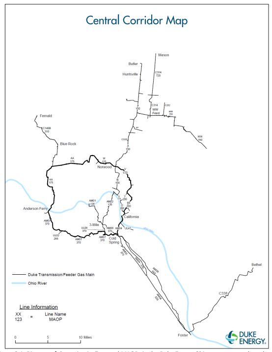
**Figure 3-1**: Diagram of the main pipelines and MAOPs in the Duke Energy Ohio system around southwest Ohio and northern Kentucky. Numbers represent the MAOP of each of the pipelines, which are identified with a letter (Line A, Line V, Line EE etc.).
