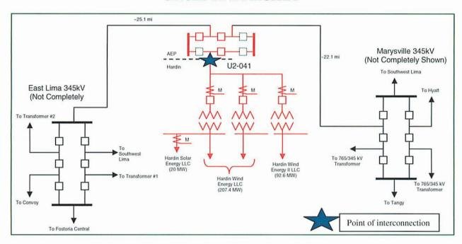
The AEP switchyard and Hardin Wind collector yard will be adjacent to each other and separated by a common fence. The Point of Interconnection will be the 345kv bus work between the two facilities with AEP owning the bus up to the deadend arrangement inside the Hardin Wind collector yard.
