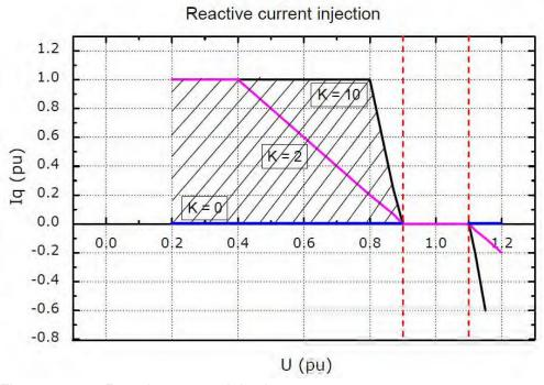
Figure 10-6: Reactive current injection
