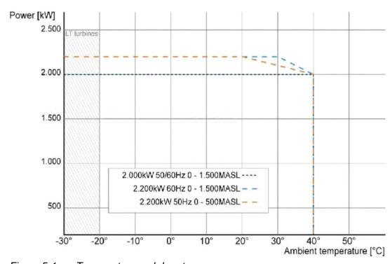
Figure 5-1: Temperature and de-rate curves
