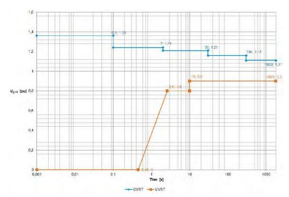
Figure 5-4: OVRT, UVRT curves for symmetrical and asymmetrical faults where  $U_{qrid}$  represents grid voltage values
