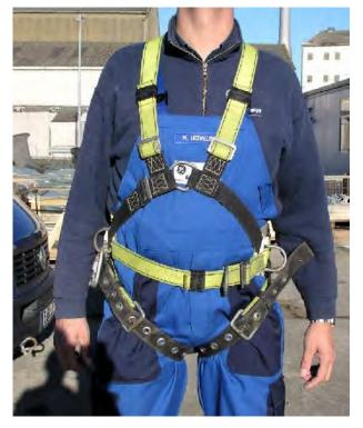
Fig. 8: Safety harness correctly fitted
