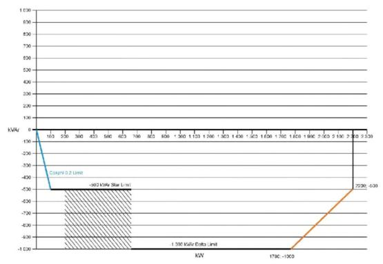
Figure 5-3: Reactive power capability for 2.2MW variants 50 and 60Hz
