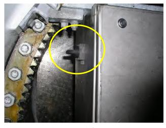
Fig. 16: Battery maintenance switch
