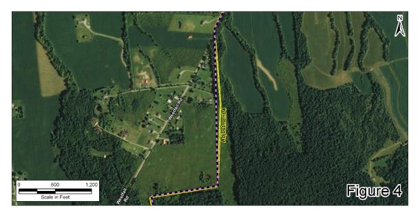
**Adjustment 5:** AEP Ohio Transco is proposing a fifth adjustment adjacent to the north of the Biers Run Substation (see Figure 5 below). The proposed adjustment is to accommodate an existing 345kV transmission line just west of the proposed alignment. Moving the transmission line pole 240 feet to the northwest, provides the necessary clearance from the existing utility. There were no changes in property owner, land use or impacts to ecological features due to this adjustment.
