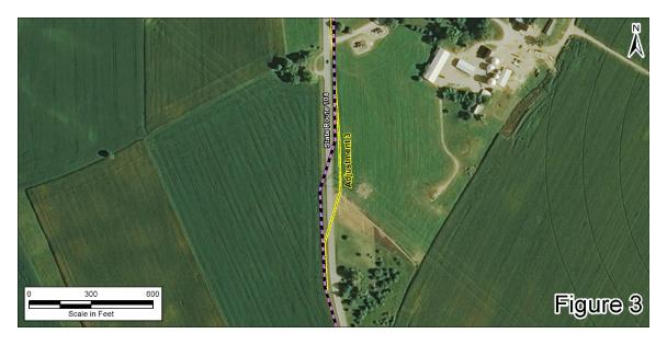
**Adjustment 4:** AEP Ohio Transco is proposing a fourth adjustment south of the Westfall Road crossing as shown on Figure 3 below. The purpose of this proposed adjustment is to optimize the span length between pole structures and to provide additional distance (and eliminate the need for multiple overhang easements) from multiple residential parcels. The proposed adjustment parallels the Certificated Route centerline approximately 75 feet east of its original placement.
