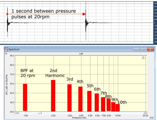
When wind turbine blades rotate past the tower a a short pressure pulse (top graphic) occurs producing a burst of infrasound.
