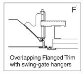
Recommended rough-in dimensions for F-trim fixtures 24"x48" (Tolerance is +1/4"-0"). Swing-gate range 1-3/16" to 3-15/16". Swing-gate span 23-3/8" to 26-11/16". Fixture swing-gate points require additional 1-1/16"over nominal fixture height.
