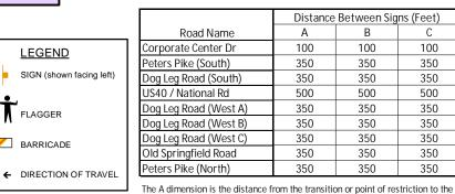
first sign. The B dimension is the distance between the first and second signs. The C dimension is the distance between the second and third signs
