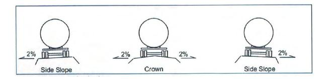
Site access roads must be constructed such that the dips or humps long the roadway do not exceed 6 inches in 50 feet. Generally it is not acceptable to double this requirement (12 inches in 100 feet) as some loads have up to and exceeding 100 feet between front and rear trailer axels with loads less than 12 inches from the road surface.
