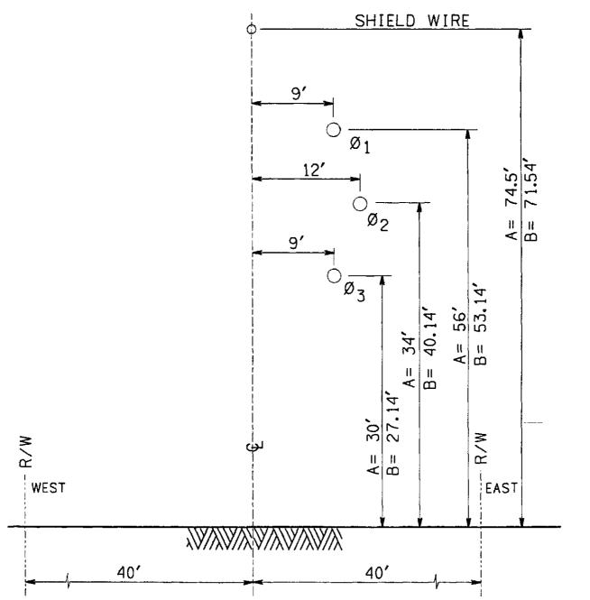
DIMENSION "A" LINE CONFIGURATION - 138KV UNDER EMERGENCY AND NORMAL MAXIMUM LINE LOADING CONDITIONS
