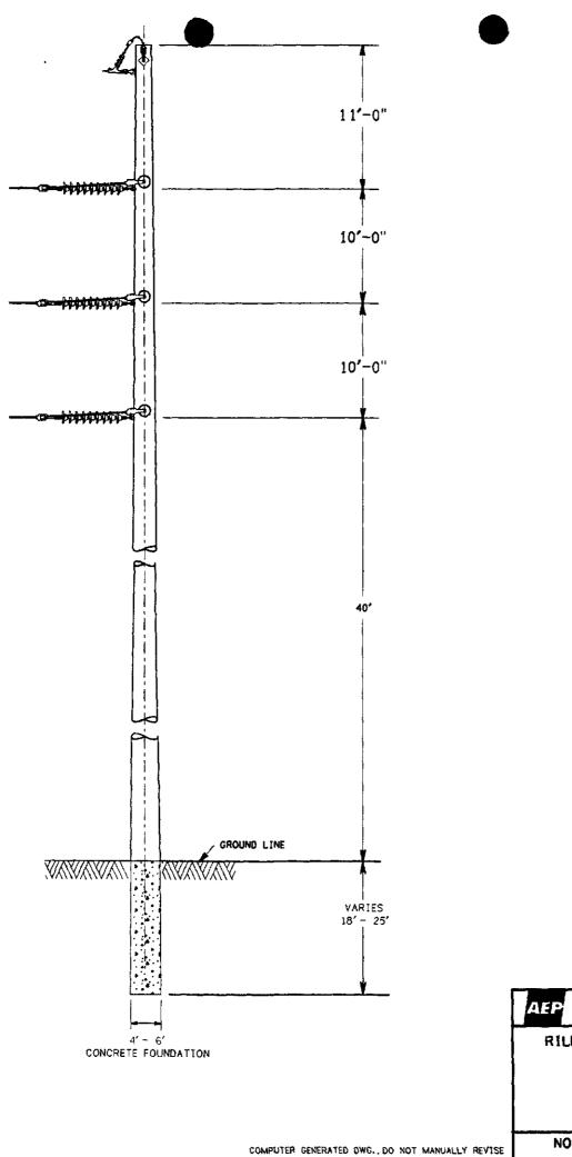
AEP AMERICAN ELECTRIC POWE RILEY CREEK - PAULDING-PUTNAM 138KV LINE SINGLE POLE STRAIN STRUCTURE 15-12(C)(6) NOT TO SCALE FIGURE 4
