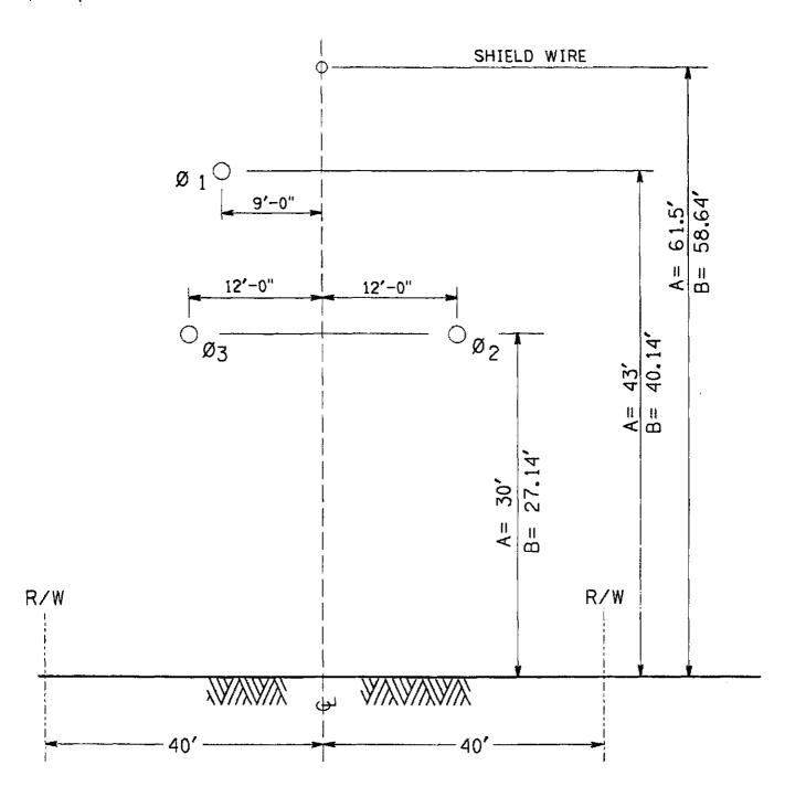
DIMENSION "A" LINE CONFIGURATION - I38KV UNDER EMERGENCY AND NORMAL MAXIMUM LINE LOADING CONDITIONS
