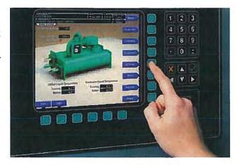
Data outputs on the OptiView Control Center are accompanied with an illustration of the appropriate chiller component, making chiller operation more intuitive.
