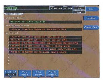
Color-coded fault messages allow early determination of chiller status and required operator action.
