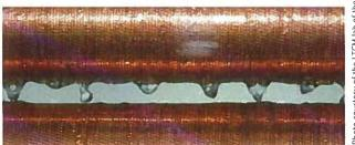
A falling-film evaporator is more efficient because refrigerant is sprayed over the tubes, reducing refrigerant charge up to 40%.
