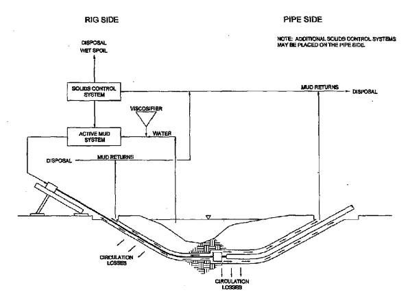
Drilling fluid expended downhole will flow in the path of least resistance. In the drilled annulus, the path of least resistance may be an existing fracture or fissure in the soil or rock substrate. When this happens, circulation can be lost or reduced. This is a common occurrence in the HDD process, but does not prevent completion. However, the environment may be impacted if the fluid inadvertently returns to the surface at a location on a waterway's banks or within a waterway or wetland.
