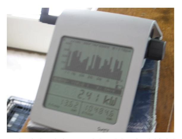
Sunnybeam data logger showing current production on 8/10/2009 of 13.62kwh for the day (10,484.6 since start up) and also graphing the values of the previous 30 days. Through a USB connection, production values are downloaded into a computer
