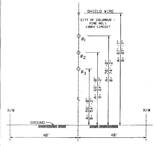
DIMENSION "A" - DOUBLE CIRCUIT - VERT. CONFIGURATION (UNDER EMERGENCY & NORMAL MAX. LINE LOADING)
