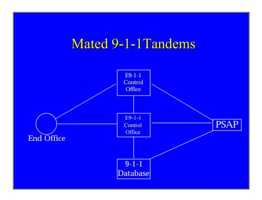
Many 9-1-1 tandems are "mated". Each end office is trunked to both tandems, and both tandems are connected to the PSAP. If one of the tandems fails, the PSAP remains in service. Call handling capacity is reduced by 50%, but there is no interruption of service.
