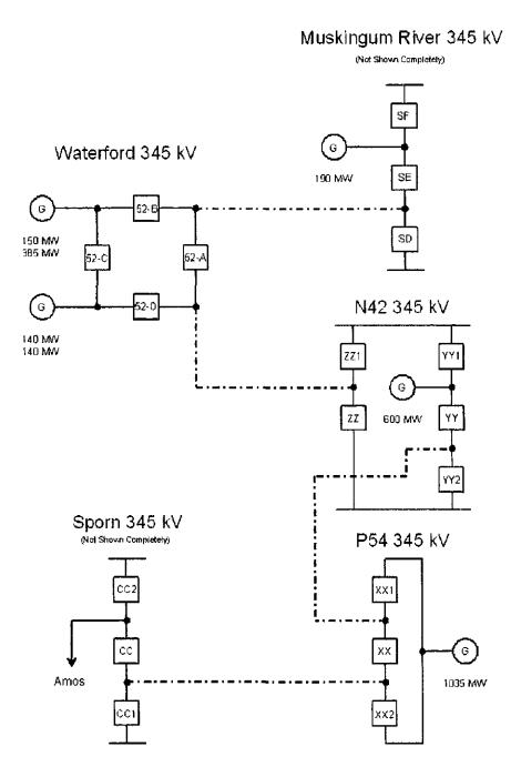
Figure 1: Anticipated future one-line switching configuration of the Sporn – Muskingum River 345 kV circuit with the PJM Project #P54 in service.
