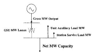
Net MW Capacity = (Gross MW Output - GSU MW Losses\* – Unit Auxiliary Load MW - Station Service Load MW)
