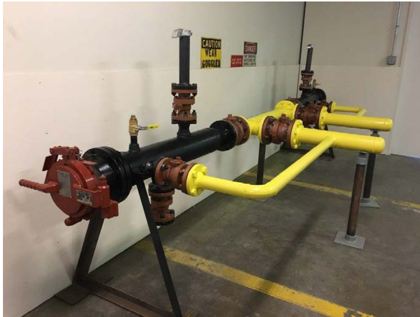
Figure 5: Pig launcher/receiver training apparatus
