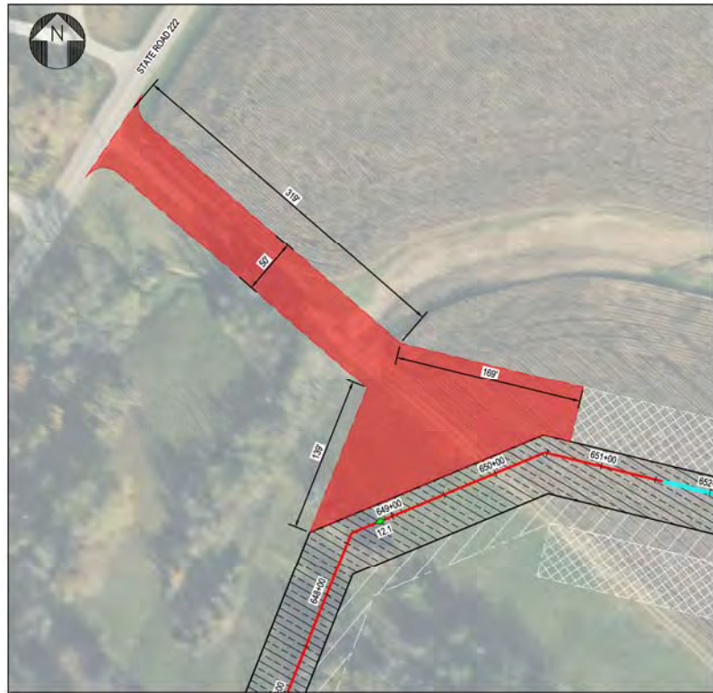
PIPELINE ACCESS PLAN 4
