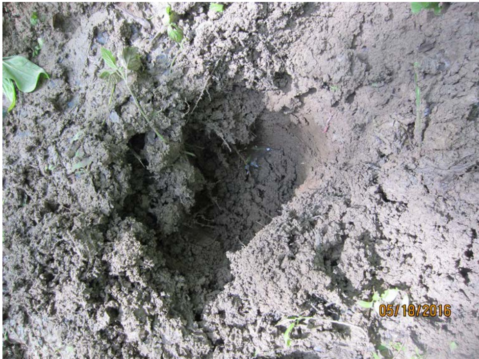
Photograph 10. View of high water table and low-chroma soil from wetland determination SP-8.
