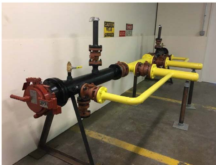
Figure 6: Pig launcher/receiver training apparatus
