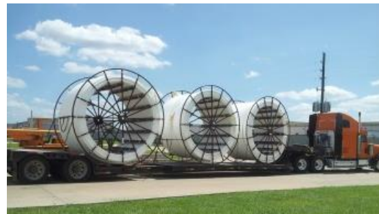
Figure 2. RTP on 12 ft OD Spools
