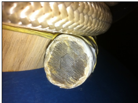
Figure 19: Braided Jacket Pulling Rope
