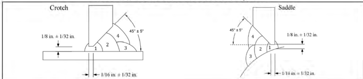
FIGURE 1 – JOINT DESIGN AND BEAD SEQUENCE
