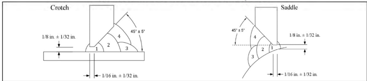
FIGURE 1 – JOINT DESIGN AND BEAD SEQUENCE
