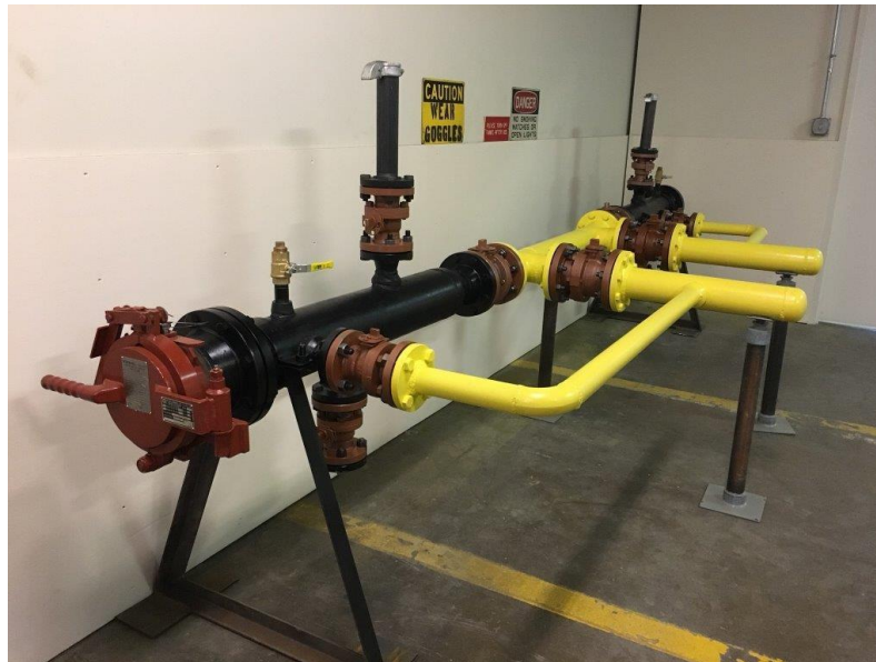
Figure 6: Pig launcher/receiver training apparatus
