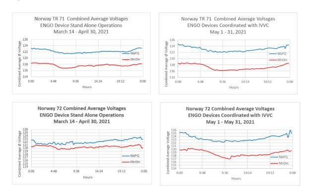
As demonstrated on the above graphs, utilizing Sentient Energy (Varentec) ENGO devices Coordinated with IVVC appears to provide improvement in terms of voltage separation and consequently CVR, especially for underperforming circuits. Further testing and study to determine optimum placement and application is required.
