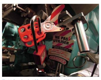
Fig. 14: Securing the HSS rotor lock with LOTO
