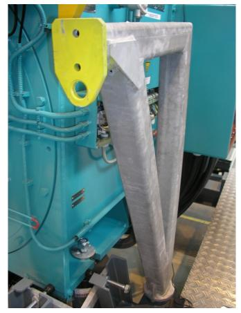
Fig. 8: Hooking point on the swinging gallows
