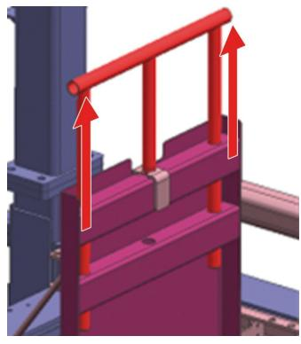
Fig. 22: Hatch converter level with extracted railing
