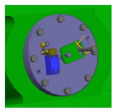
Fig. 18:: Securing the rotor lock - Cypress turbines
