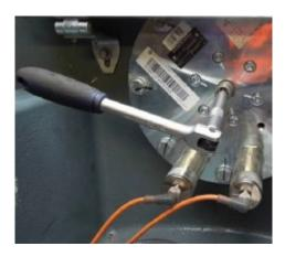
Fig. 16: Mechanical rotor lock actuation
