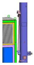
Fig. 25: Hatch bar placed at the console column
