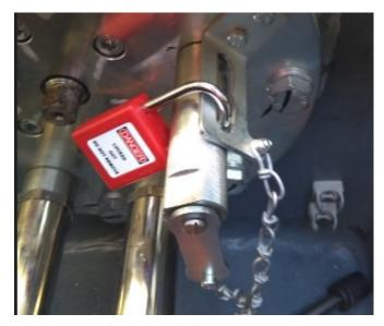
Fig. 17: Securing the LSS rotor lock - 3 MW
