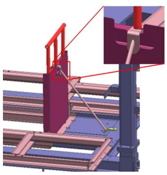
Fig. 23: Locking the railing with the hatch bar
