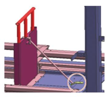
Fig. 24: Bolting the hatch bar to the console
