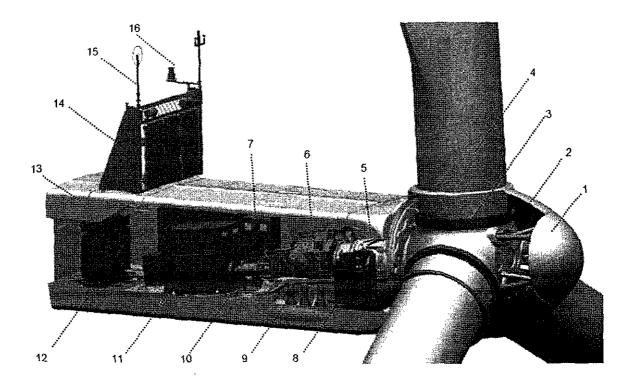
1 Rotor cover 9 Yaw system 2 Pitch system 10 High speed shaft 11 Generator 3. Blade bearings 12 Transformer 4 Blades 5 Low speed shaft 13 Nacelle cover 14 Cooling system 6 Gearbox 15 Wind sensors 7 Electrical cabinets 8 Hydraulic group 16 Beacon system
