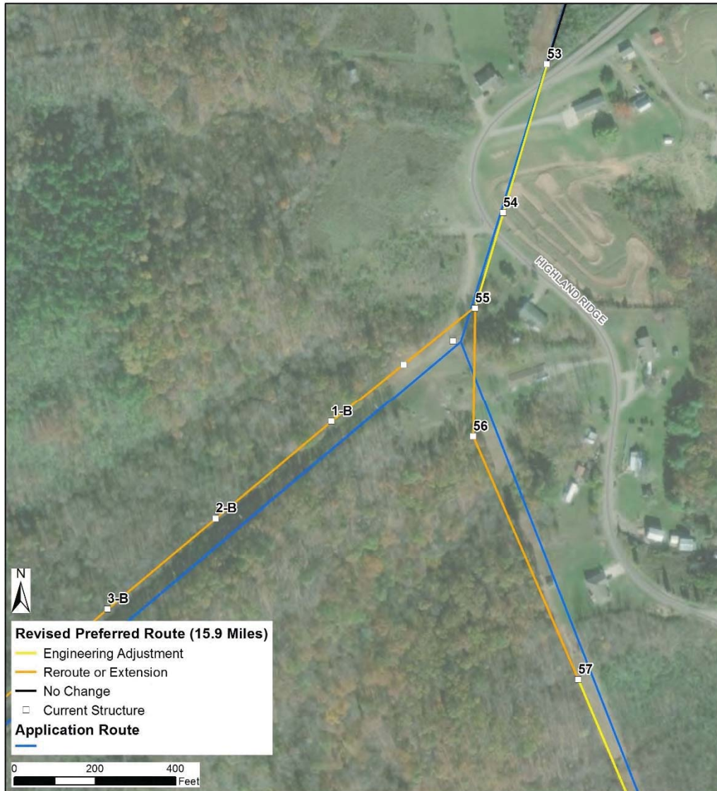
Exhibit 5. Map Illustration of Engineering Adjustment (Structures 53 through 55)
