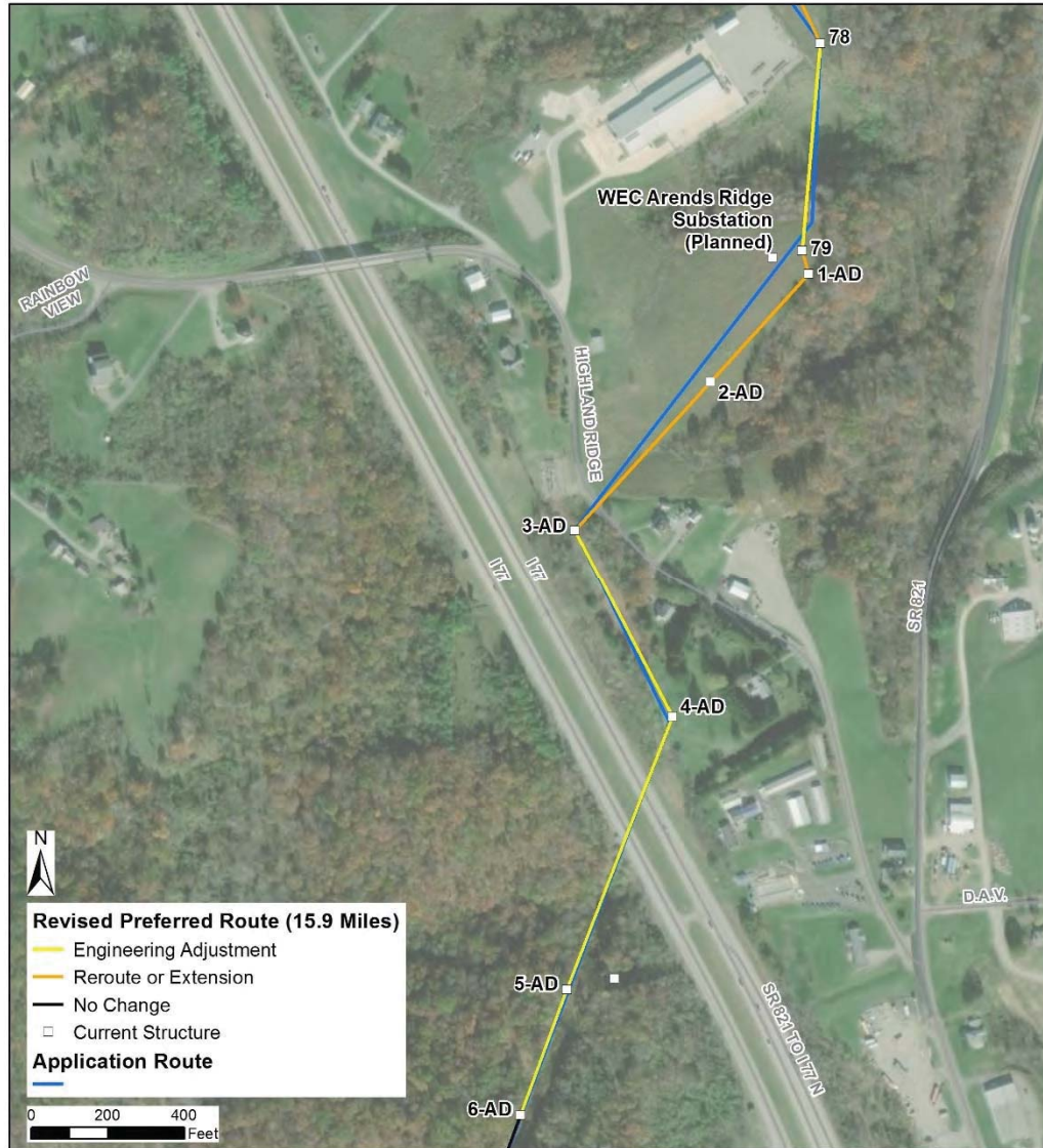
Exhibit 11. Map Illustration of Engineering Adjustment (Structures 78 through 79)
