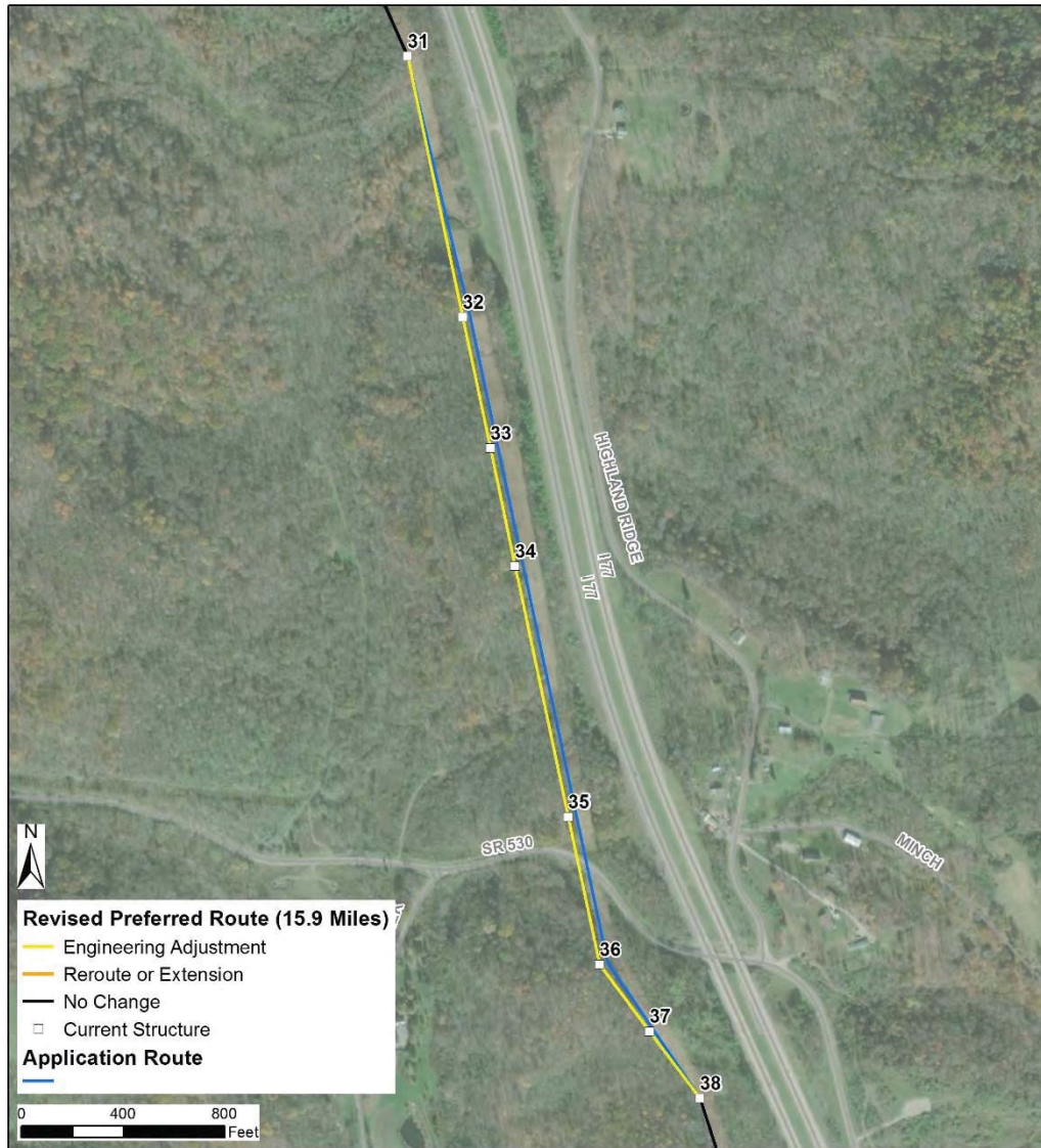
Exhibit 4. Map Illustration of Engineering Adjustment (Structures 31 through 38)
