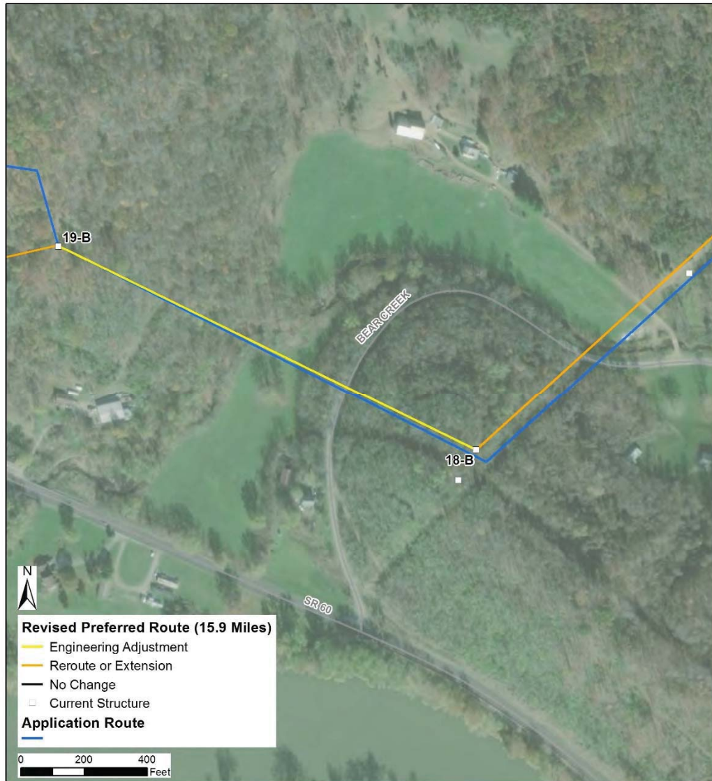
Exhibit 8. Map Illustration of Engineering Adjustment (Structures 18-B through 19-B)
