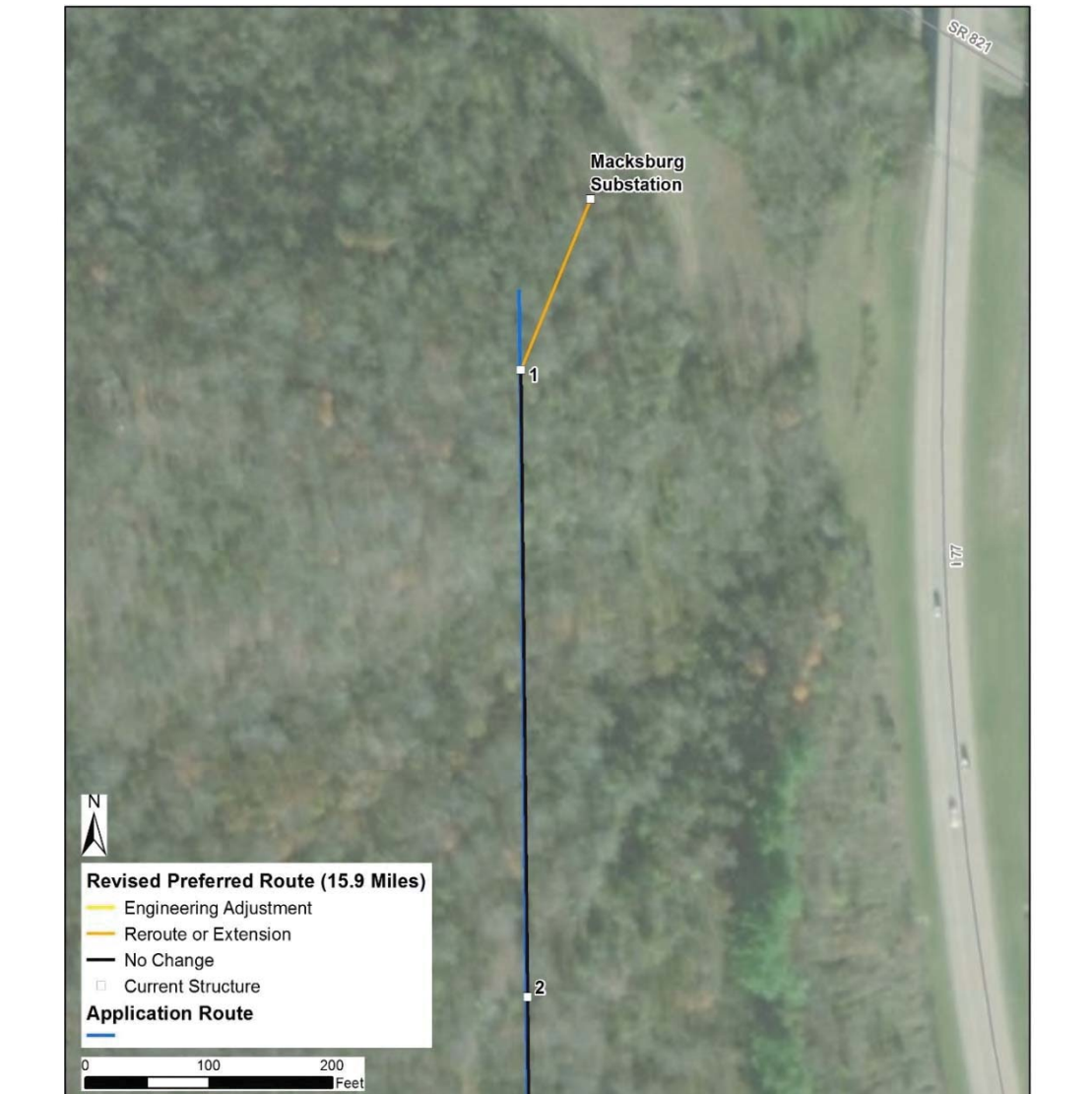
Exhibit 12. Map Illustration of Reroute 1 (Structures Macksburg Substation and Structure 1)
