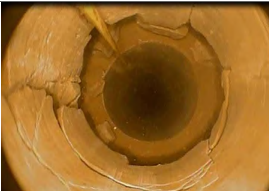
GEO-066, 8:16 31 ft, "void" identified in geotechnical boring
