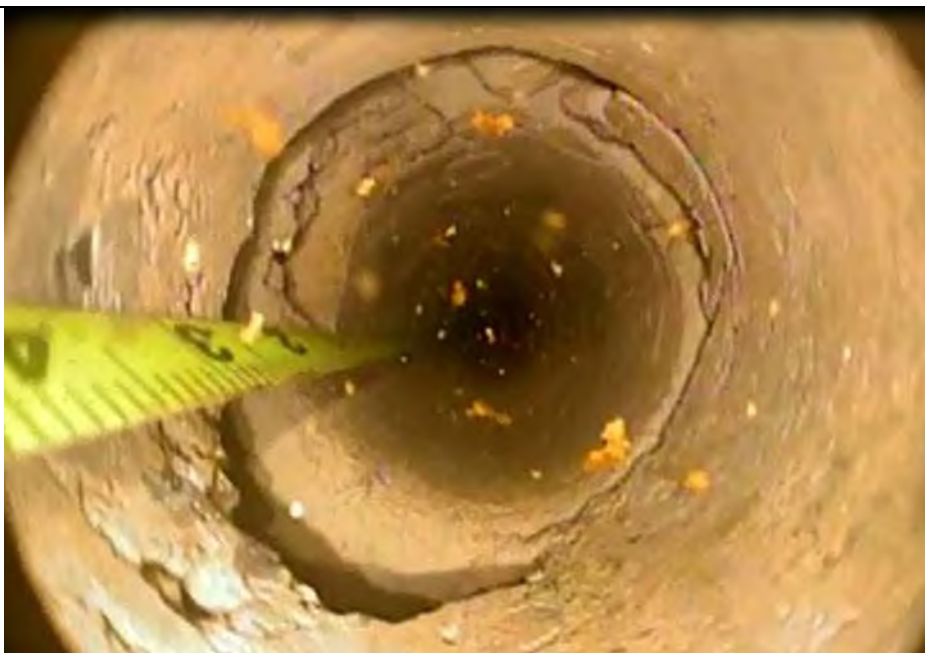
GEO-096, 14:28 42.5 ft, near where drilling fluid circulation was lost, small opening with some missing limestone pieces
