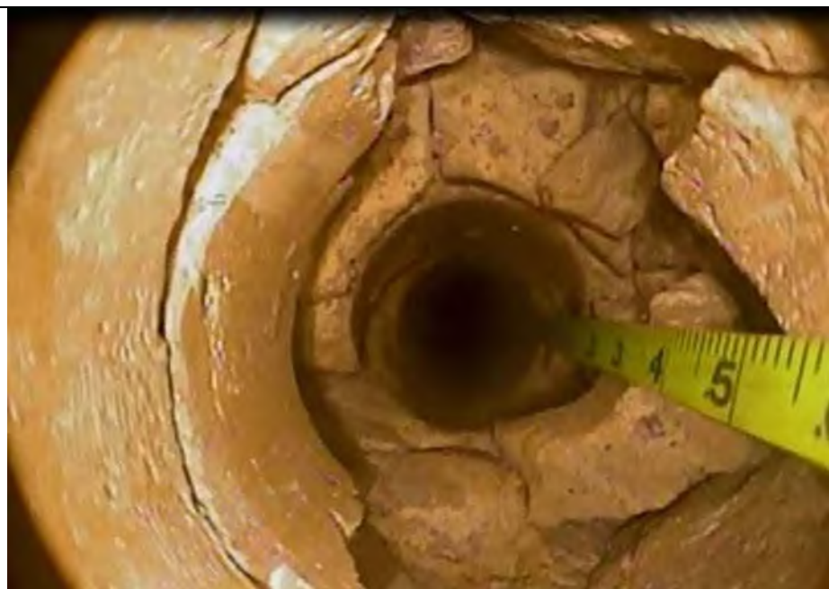
GEO-086, 3:21 15.5 ft, highly fractured, rugged borehole with pieces missing, near depth where drilling fluid circulation was lost
