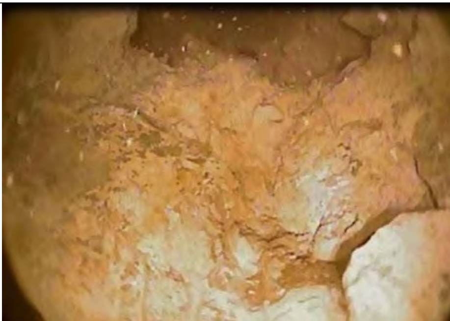
GEO-047, 13:50 58 ft, view of sidewall of “void”, rugged dissolution features, had back
