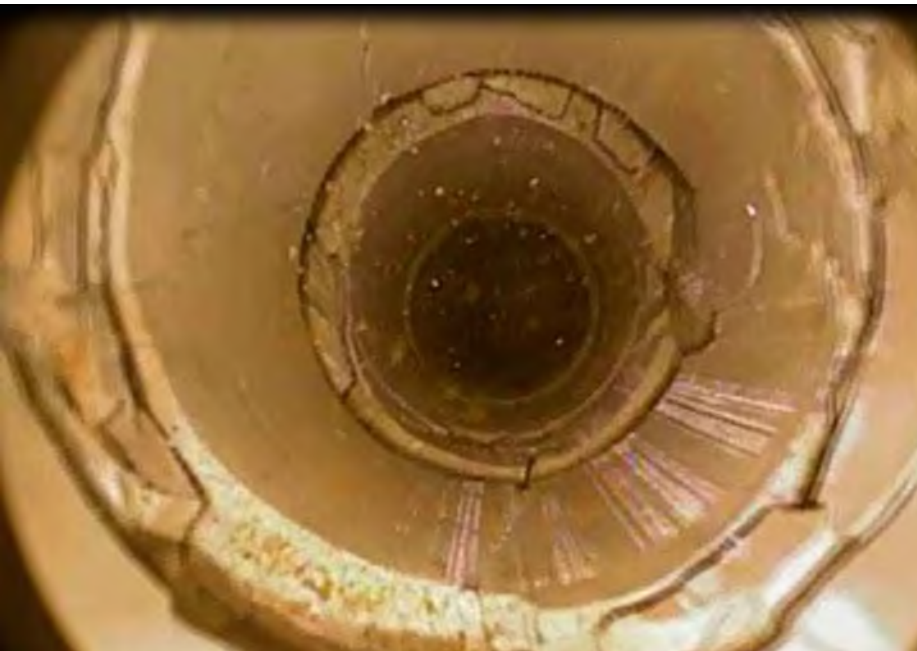
GEO-047, 4:20 Typical borehole in upper 40 feet. Fractures and small openings have backs
