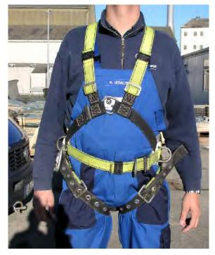
Fig. 8: Safety harness correctly fitted
