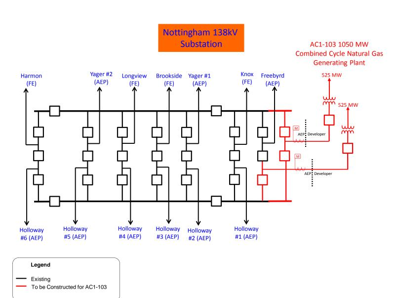
Figure 2: Point of Interconnection (Nottingham 138 kV Substation)
