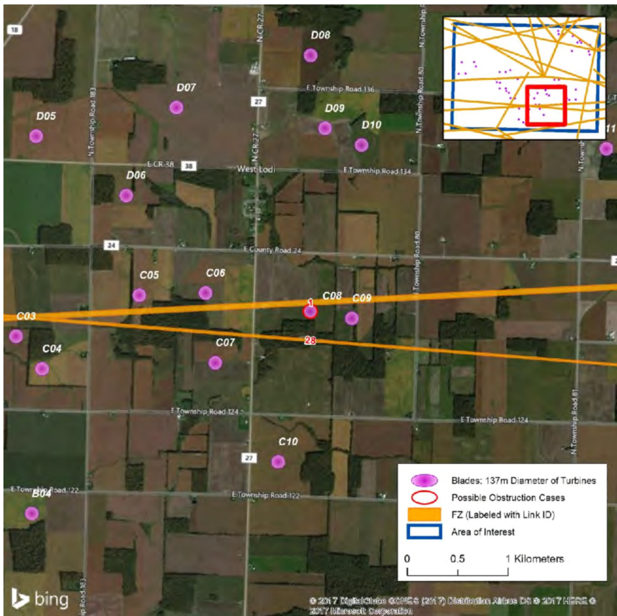
Figure 4: Potential Obstruction Case with Turbine C08
