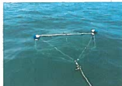
Photo 3. Larval fish monitoring using the neuston net.
