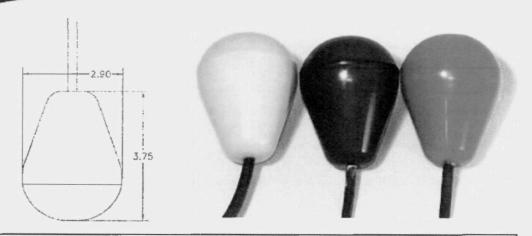
Normally Open (N/O): Pump duty. As the float raises 1" (5º) above horizontal, the contact becomes closed and completes the circuit. This float is generally used to turn on pumps.
