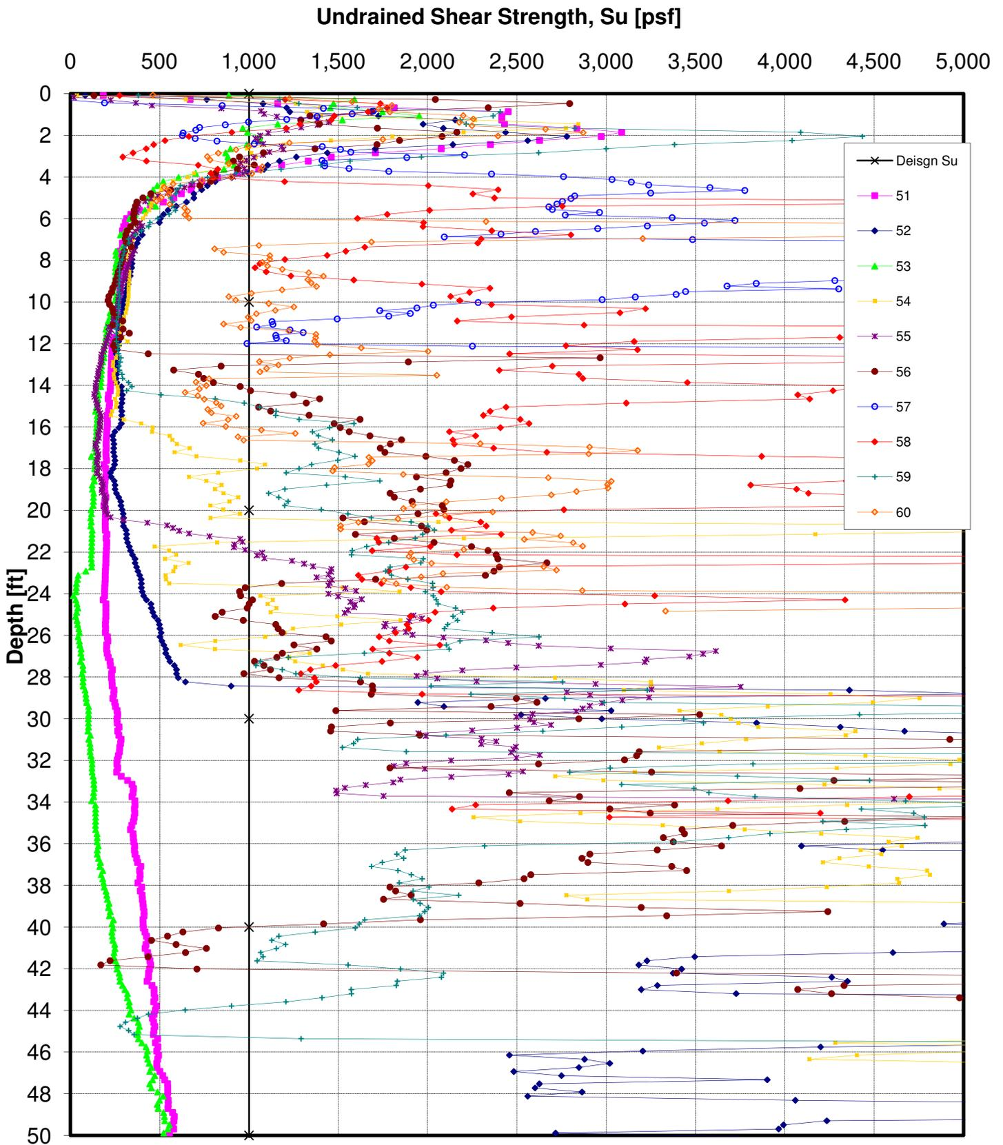
**Figure 18. Undrained Shear Strength from CPT vs. Depth Turbines 51-60**
