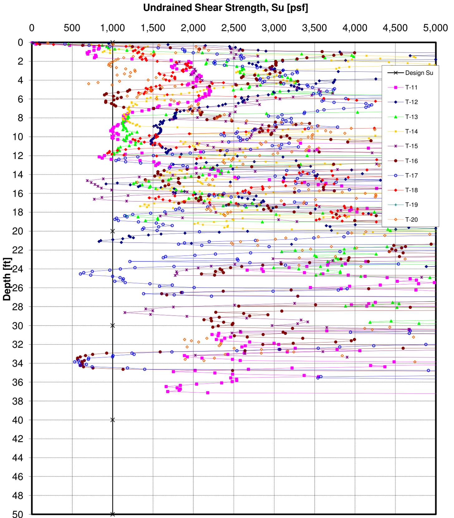
**Figure 14. Undrained Shear Strength from CPT vs. Depth Turbines 11-20**
