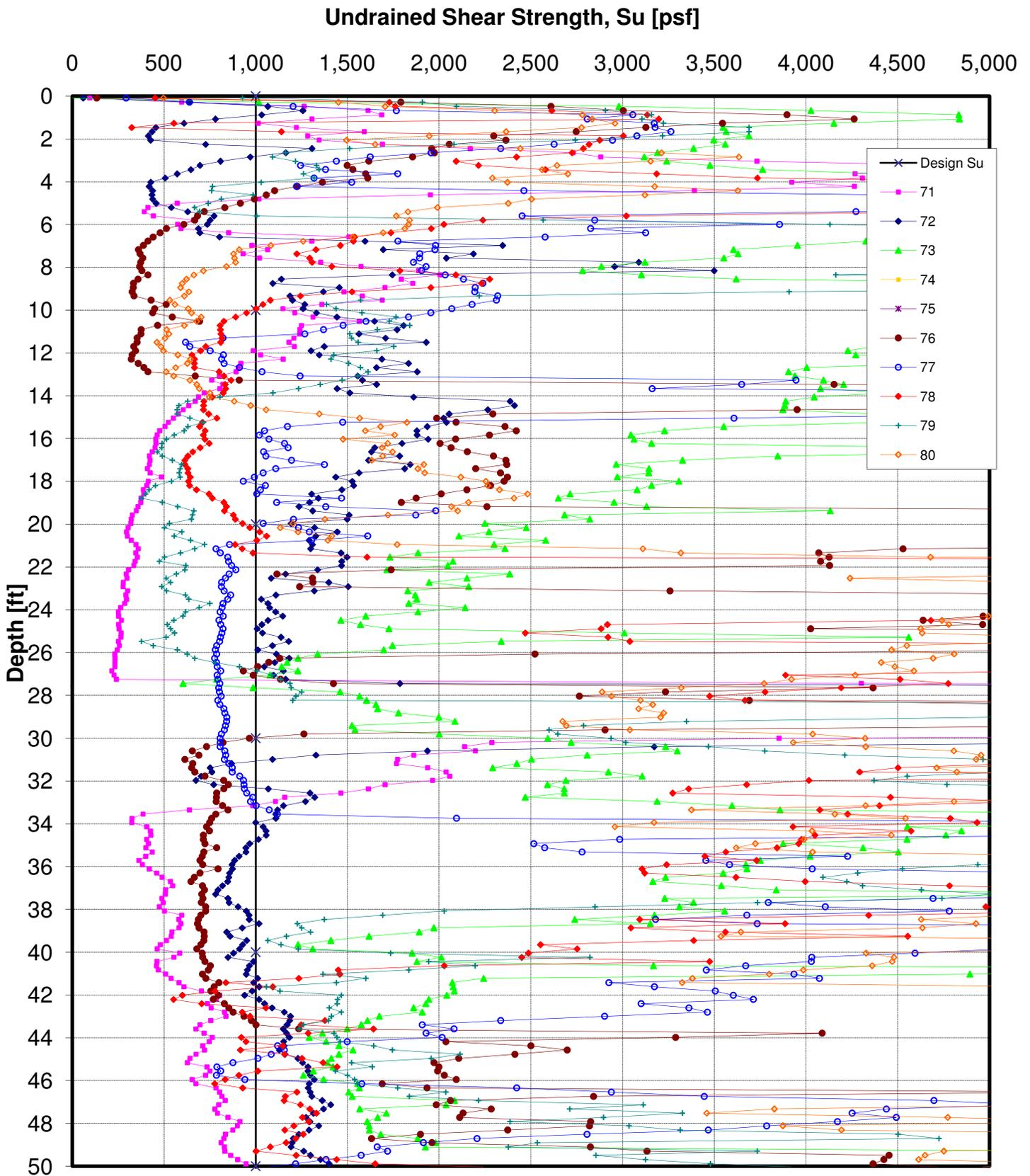
Figure 20. Undrained Shear Strength from CPT vs. Depth Turbines 71-80
