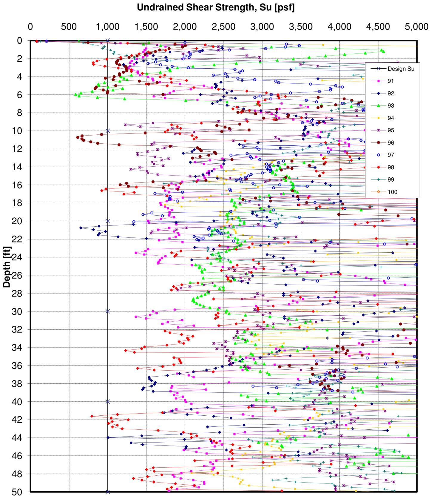
Figure 22. Undrained Shear Strength from CPT vs. Depth Turbines 91-100
