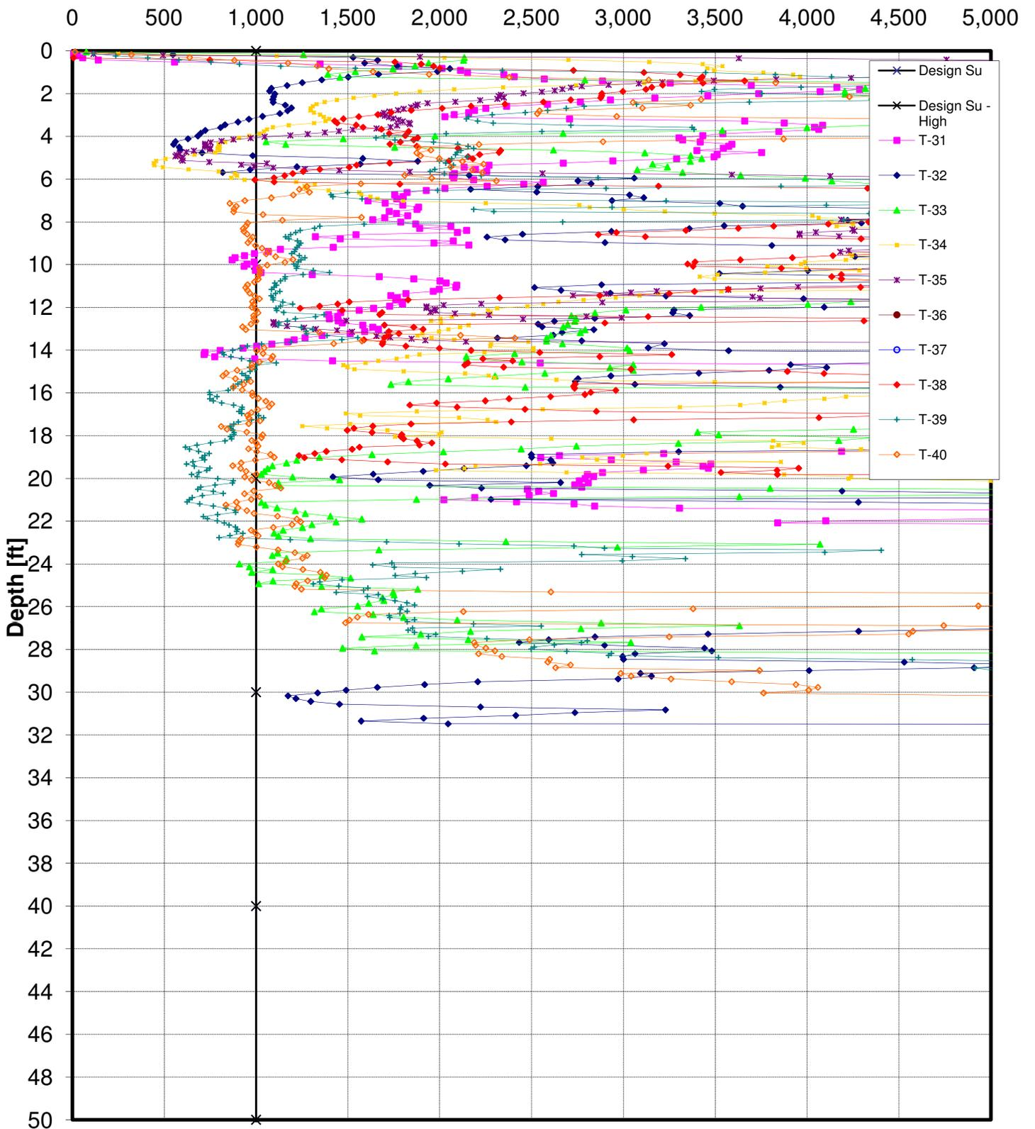
Figure 16. Undrained Shear Strength from CPT vs. Depth Turbines 31-40
