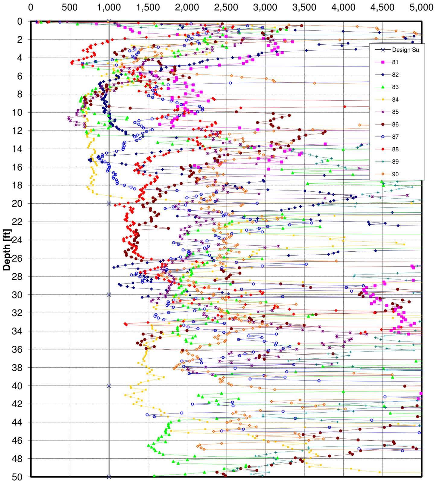
Figure 21. Undrained Shear Strength from CPT vs. Depth Turbines 81-90
