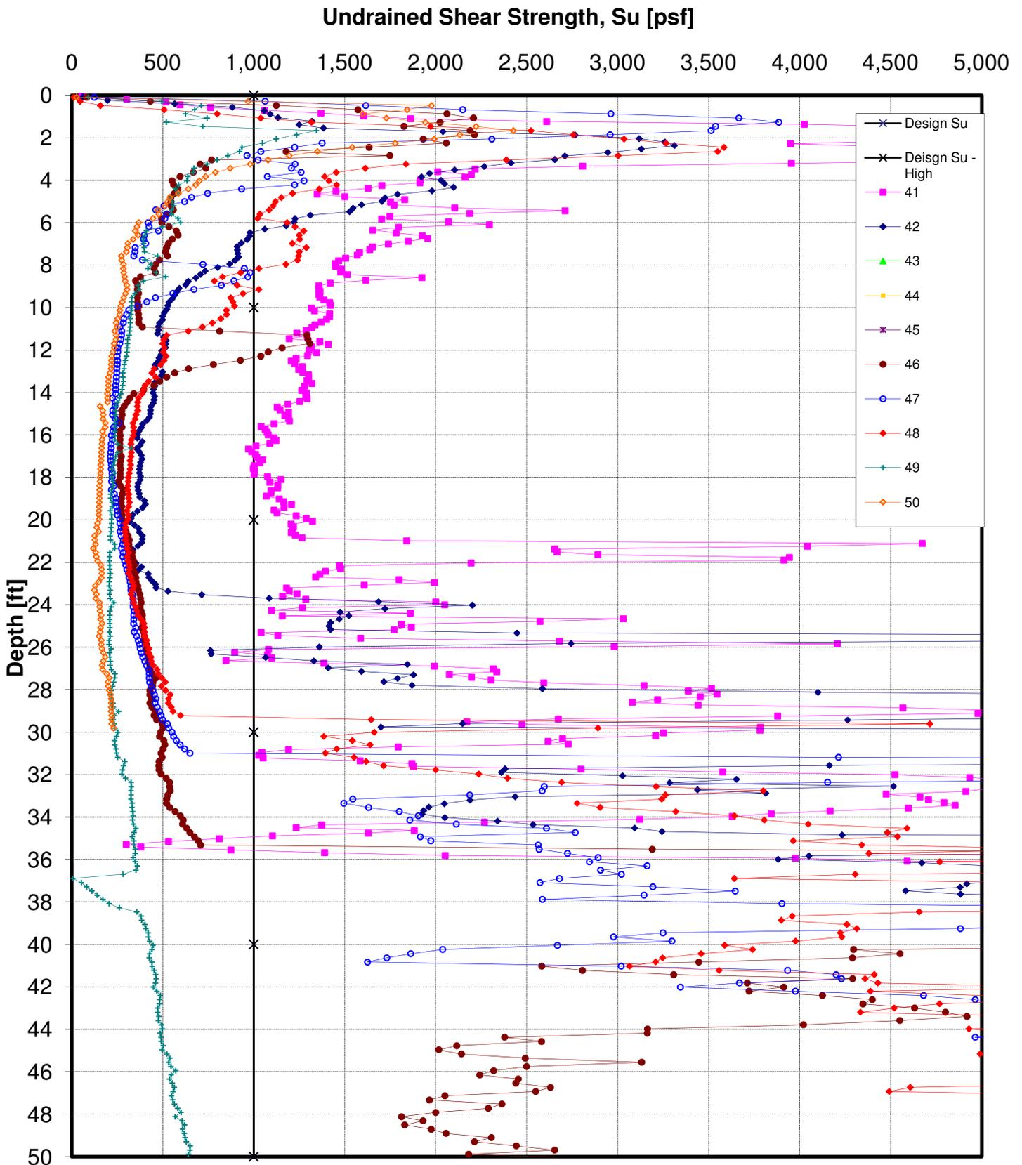
**Figure 17. Undrained Shear Strength from CPT vs. Depth Turbines 41-50**
