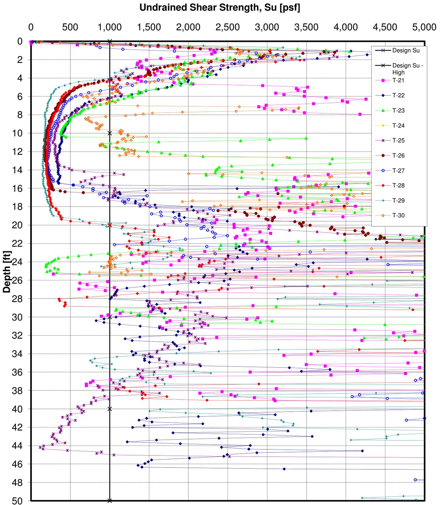
Figure 15. Undrained Shear Strength from CPT vs. Depth Turbines 21-30
