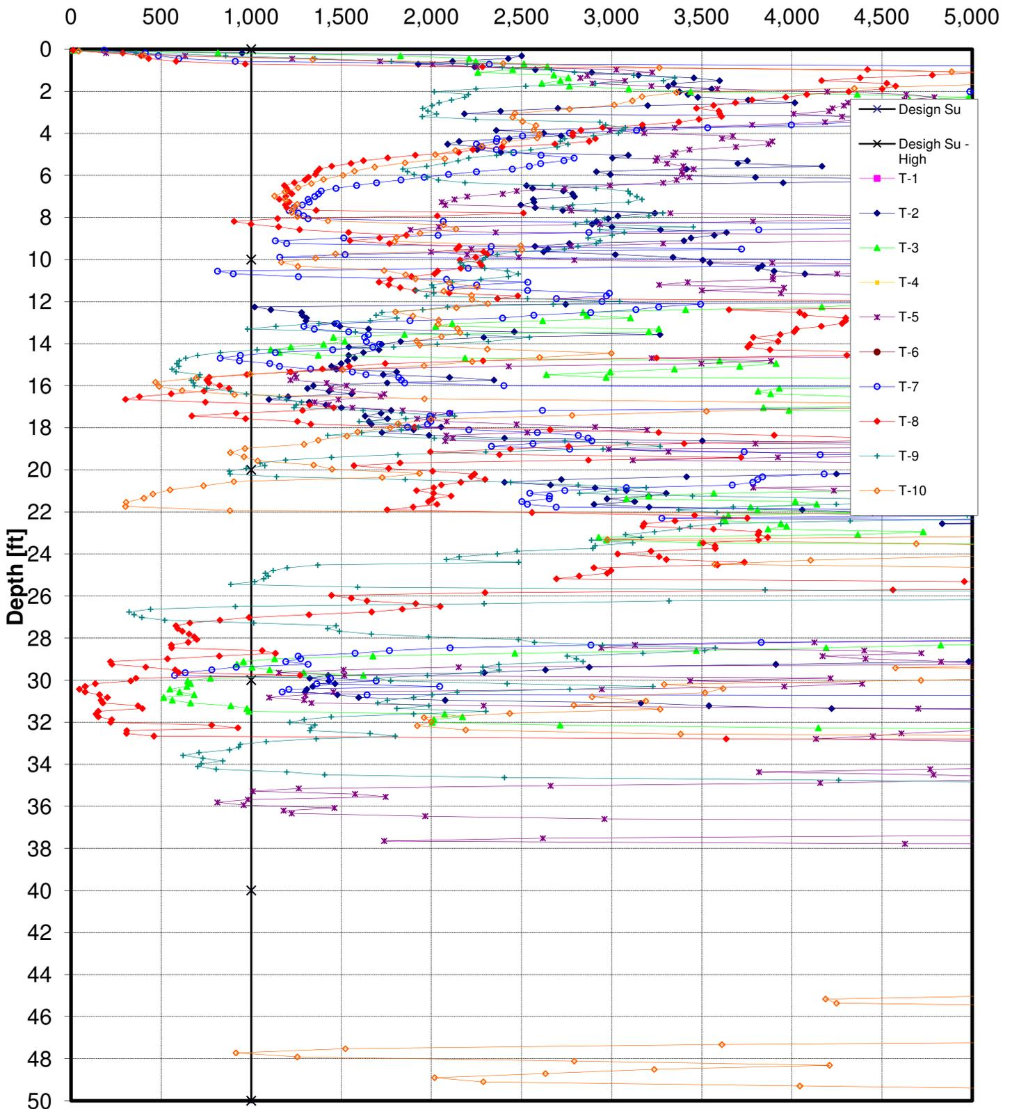
Figure 13. Undrained Shear Strength from CPT vs. Depth Turbines 1-10
