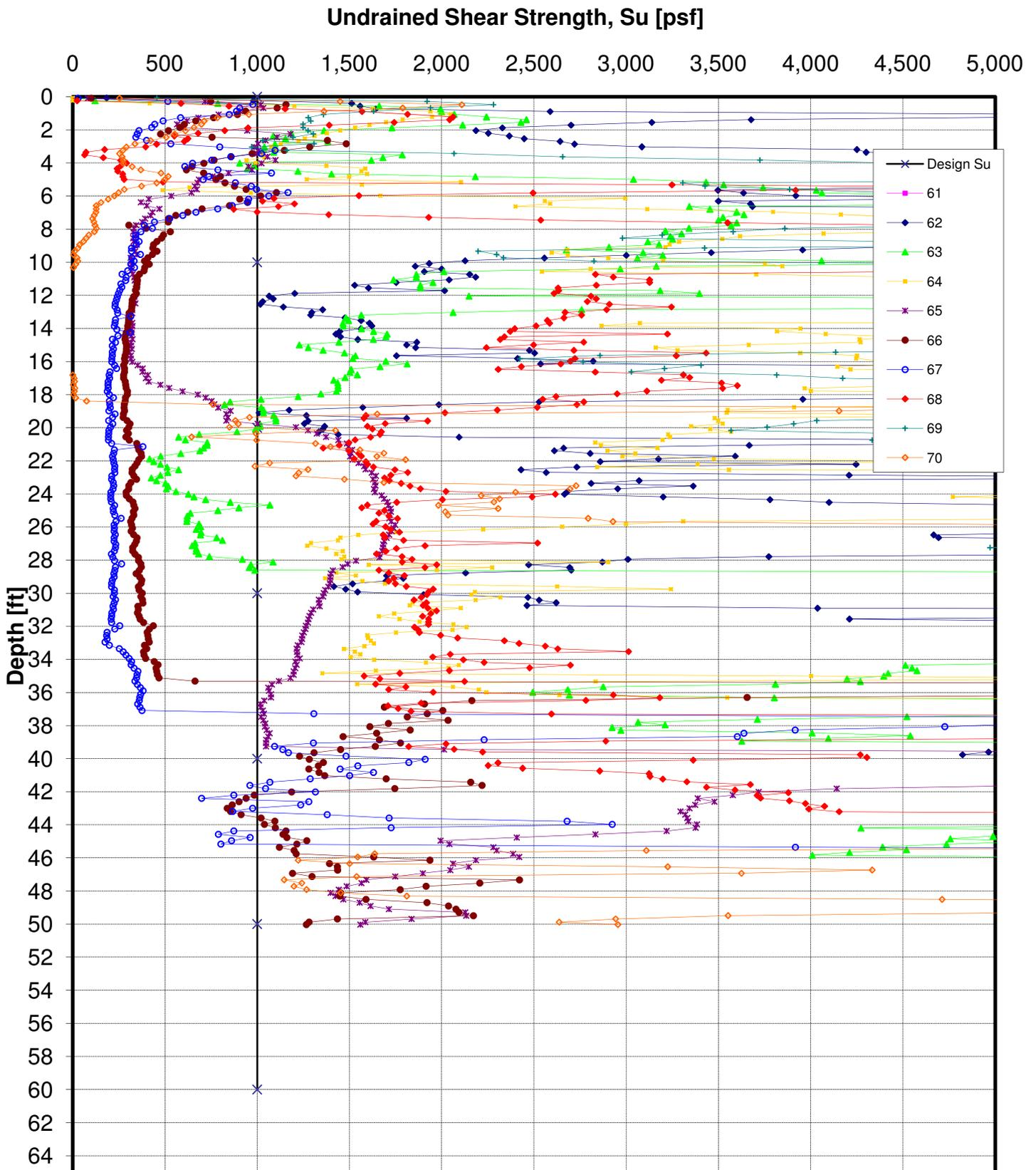
**Figure 19. Undrained Shear Strength from CPT vs. Depth Turbines 61-70**
